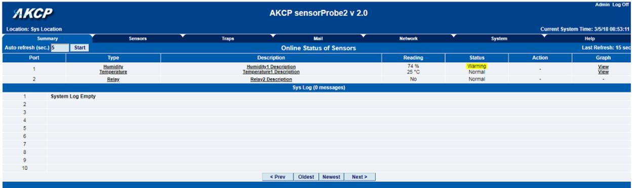
The screenshot shows the 'Online Status of Sensors' page. It features a table with columns for Port, Type, Description, Reading, Status, Action, and Graph. Two sensors are listed: Humidity (Port 1) and Relay (Port 2). The Humidity sensor shows a 74% reading and a 'Warning' status. Below the table is a 'Sys Log (0 messages)' section with a list of log entries (1-10) and navigation buttons for 'Prev', 'Oldest', 'Newest', and 'Next'.
